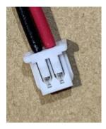
The standard way of putting the Positive and Negative (Red and Black) into the Molex Pico blade when you are putting it on a battery as a power source is like this in this picture.
