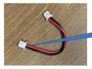
This end should go in the dongle. It is the one that is wired the nonstandard way. See below
