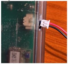
that is used for single cell LiPo batteries that also has the same style 1.25mm Pico Blade connection.
